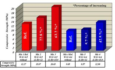
Figure 3. The influence of copper fibers to strengthen pure gypsum mixtures through the aspect ratio (for two different diameters) and the water/gypsum ratio
