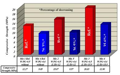
Figure 4. Effect of variable aspect ratios and W/G ratio at compressive strength of the mixture
